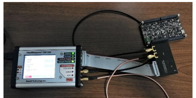
Figure 8 Picture of a RAMN board connected to ChipWhisperer Pro through a dedicated expansion board.
