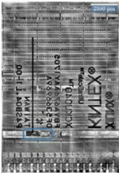
Figure 7: Overview reflected light image of the Xilinx Ultrascale XCKU040 die. The area containing the configuration and decryption logic is highlighted.
