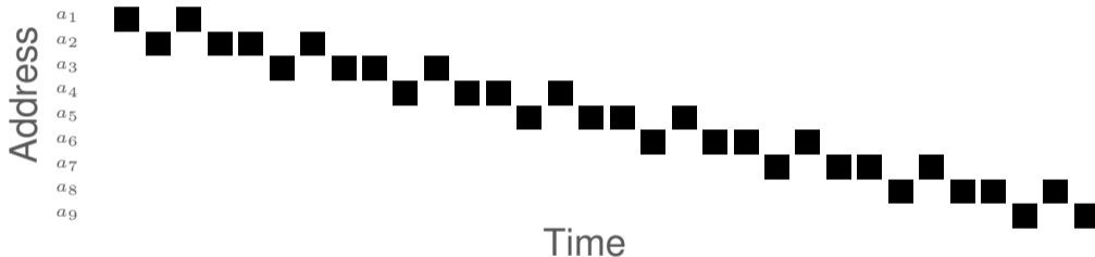
Figure: Fast and effective on Haswell. Eviction rate >99.97\% .
