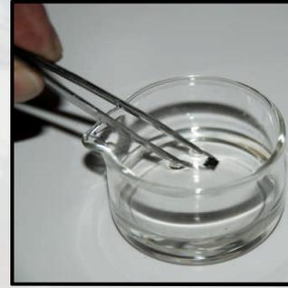
Chip is cleaned with acetone (40°C)
