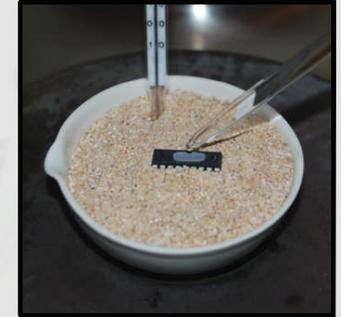
Nitric acid is dropped on chip at 50-90°C
