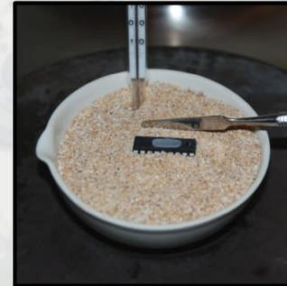
Chip is placed in heated laboratory sand bath
