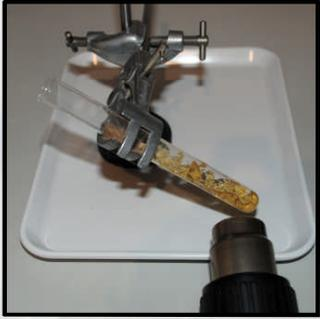
Colophony is heated near to boiling point (250-350°C)
