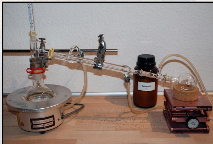
Standard distillation apparatus
