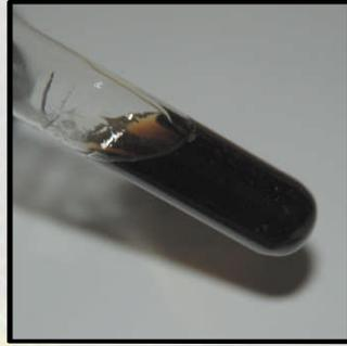
Chip package dissolves in heated liquid (5-20 min)
