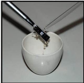
Remains of acid are removed with acetone
