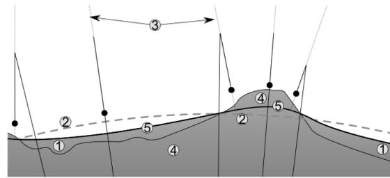
Figure 2: Figure of the Geoid. 1 ocean, 2 ellipsoid, 3 local plumb-line, 4 continent, 5 geoid.
