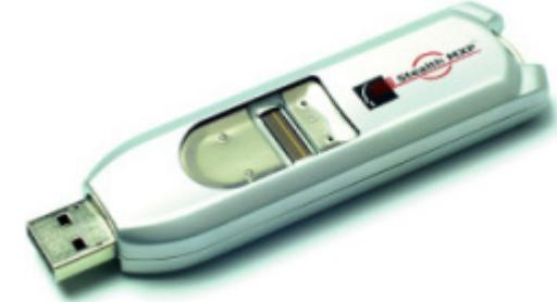
Passwords are injected upon creation from the external USB interface. A random salt is also injected as plain text through the USB interface and stored in EEPROM. The password is combined with the salt, then hashed using the SHA256 algorithm and stored in EEPROM associated with the user. The password is then deleted from memory. Password authentication and verification is done by
