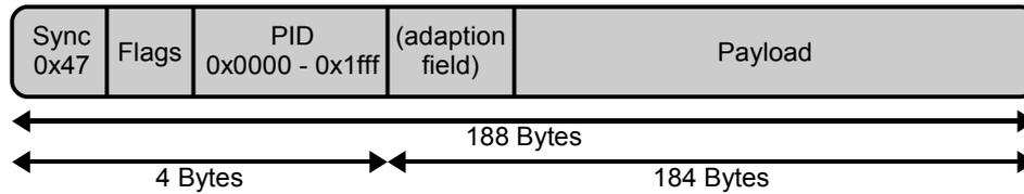
Figure 6: ISO/IEC-13818-1 Transport Stream packet header
