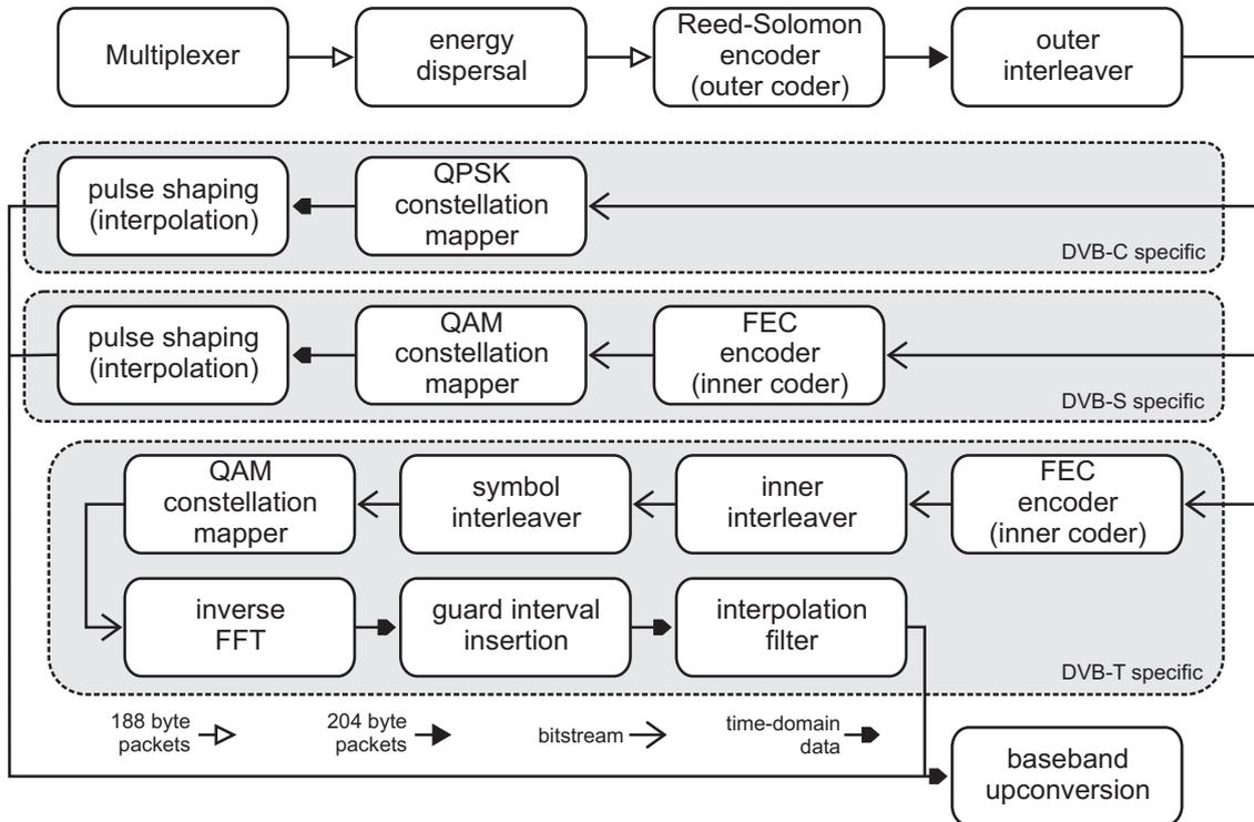
Figure 7: DVB modulator data flow
