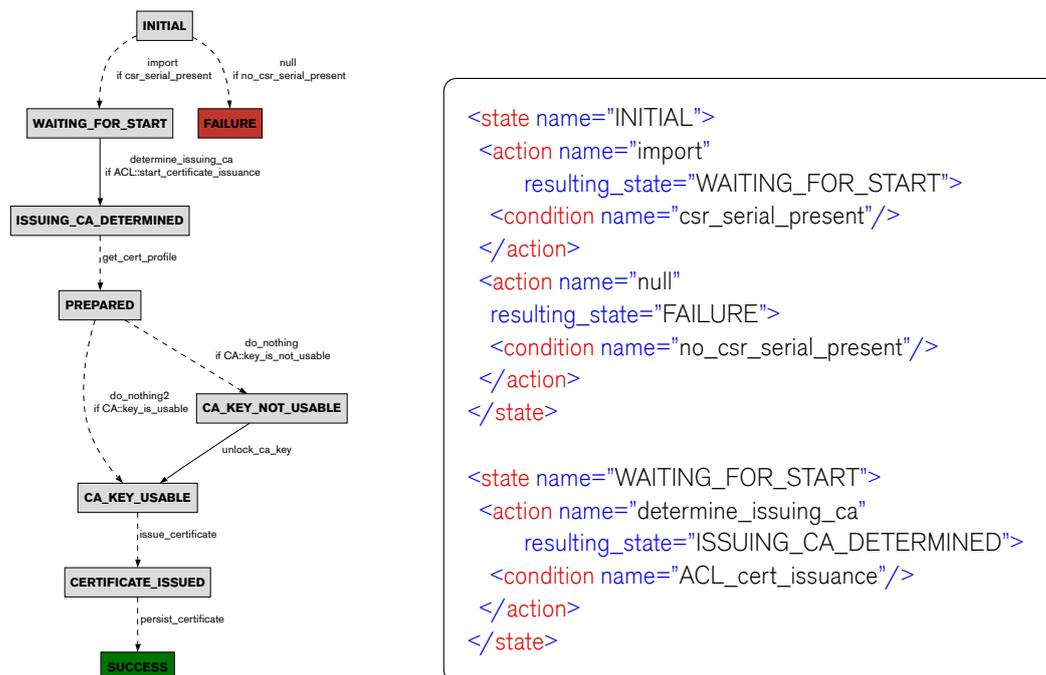
Figure 1 Graphviz rendering and a snippet from the XML definition
