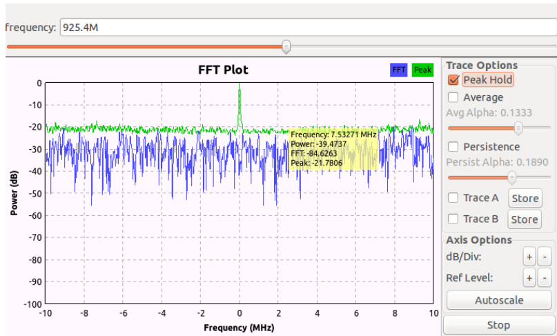
Figure 6: FFT sink showing a station channel jammed by our transmitter
